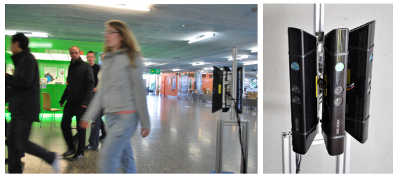
Fig. 4. The setup consisting in three vertically mounted Kinect sensors offering a joint field of view of 130^\circ \times 50^\circ and supplying RGB-D data with a resolution of 1440 \times 640 pixels at 30 \text{ Hz} . They are mounted at 1.2 \text{ m} height.
